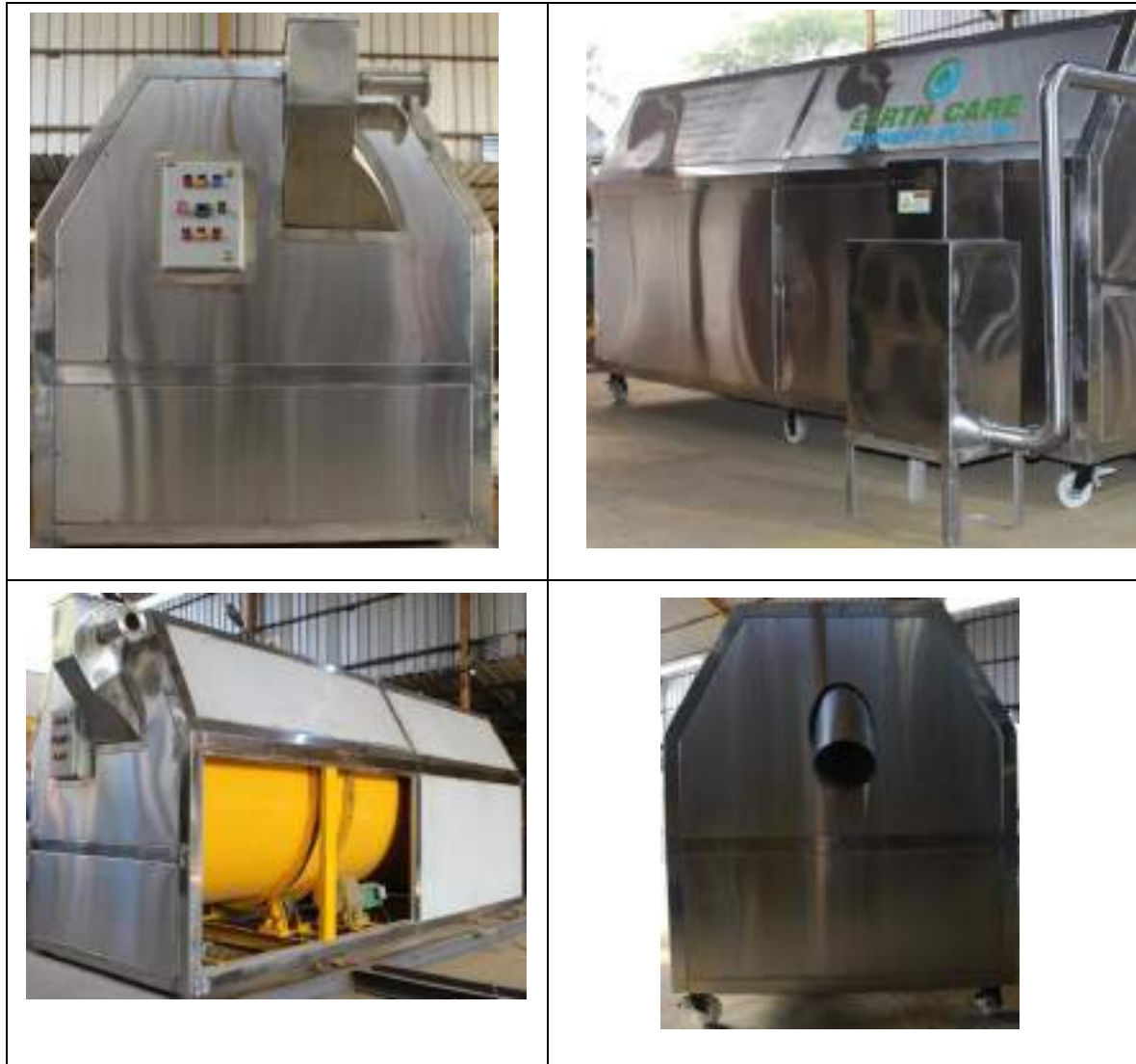
Figure 17: Typical Organic Waste Converter
