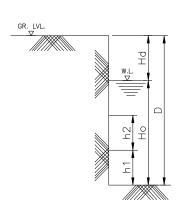
Three sets of observations shall be made and the average value of Hd is determined. Immediately on completion of borehole, Record of Boring shall be prepared and submitted to the Engineer in triplicate.
