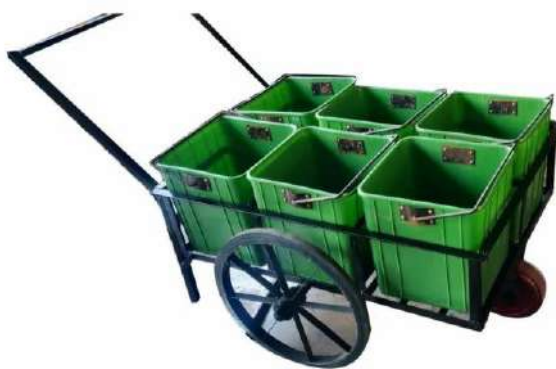
Figure 8: Handcart for collection of MSW from slum areas
