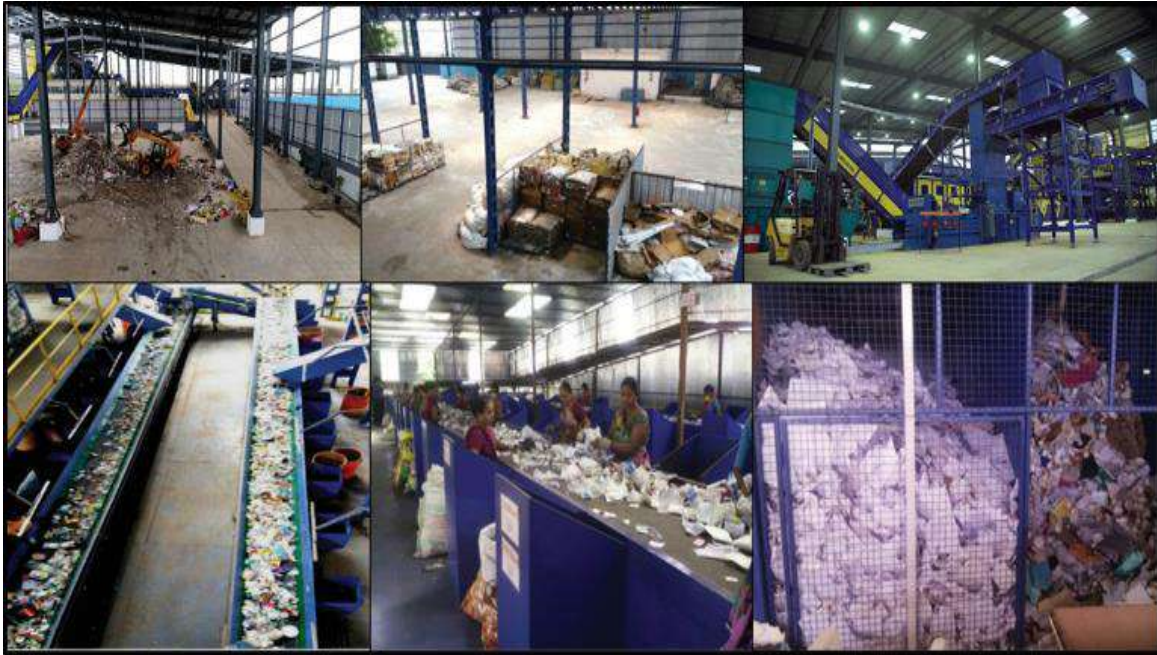
Figure 14: Operations at a typical Automated Material Recovery Facility
