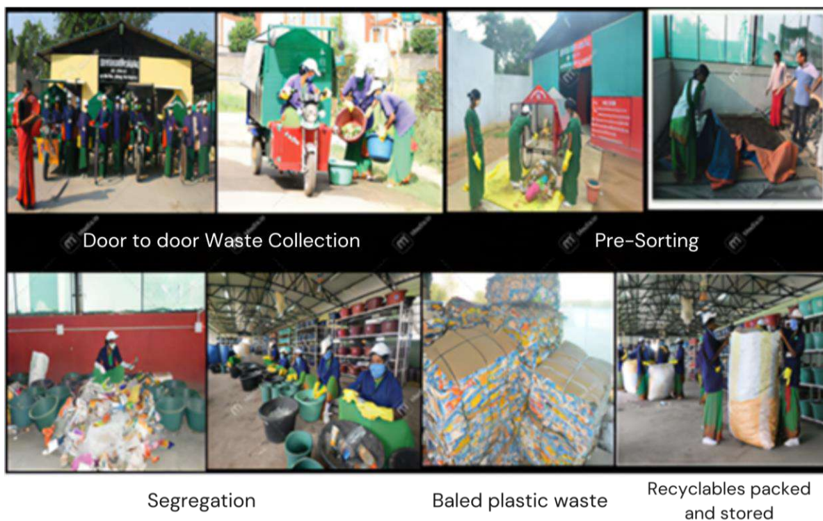
Figure 12: Activities in Manually Operated MRF
