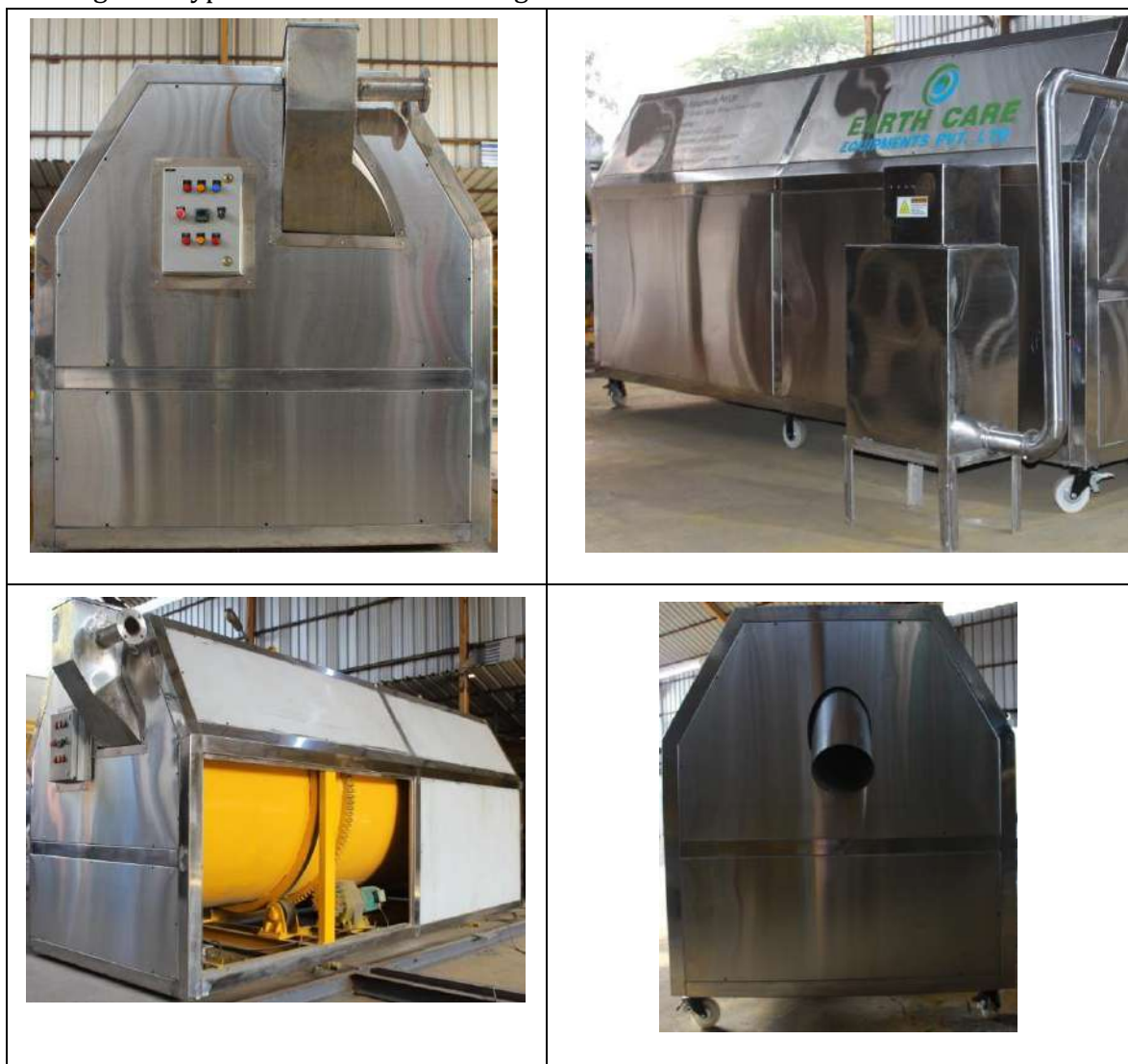
Figure 17: Typical Organic Waste Converter
