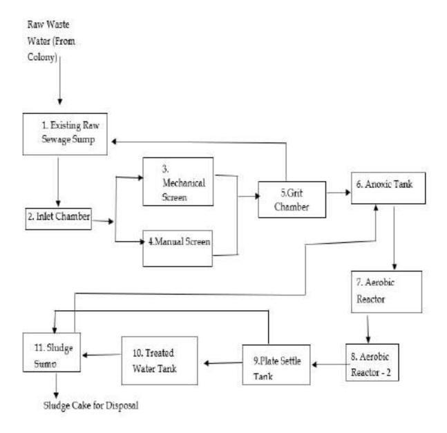
Figure 17: Process flow diagram of Gopalpuri STP
