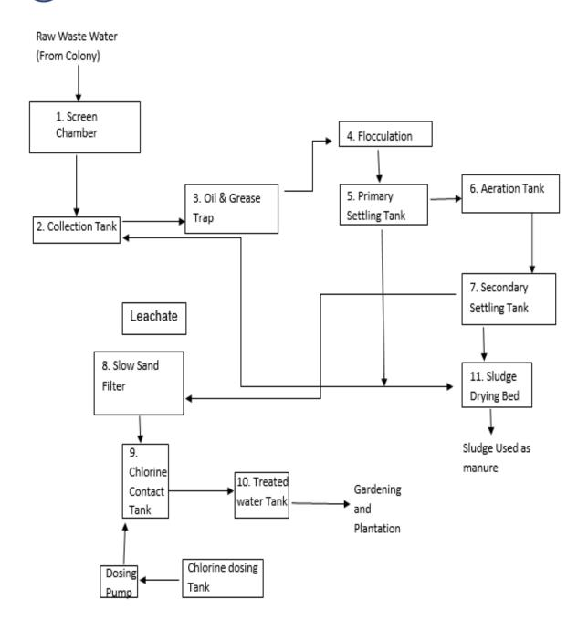
Figure 16: Process flow diagram of Kandla STP
