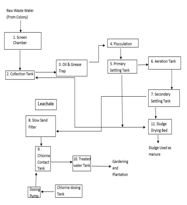
Figure 16: Process flow diagram of Kandla STP
