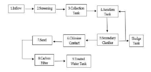
Figure 18: Process flowchart for the Vadinar STP
