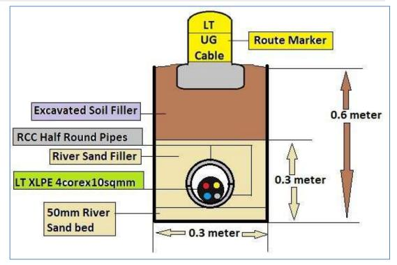
The site requirement & position of fixing the markers will be decided by the Engineer-Incharge or his nominee. The type of route marker & letters to be written on the route marker will be decided while execution by the Engineer-in-charge. Route marker should be visible and the pedestal should be buried underneath the ground firmly by providing CC foundation.
