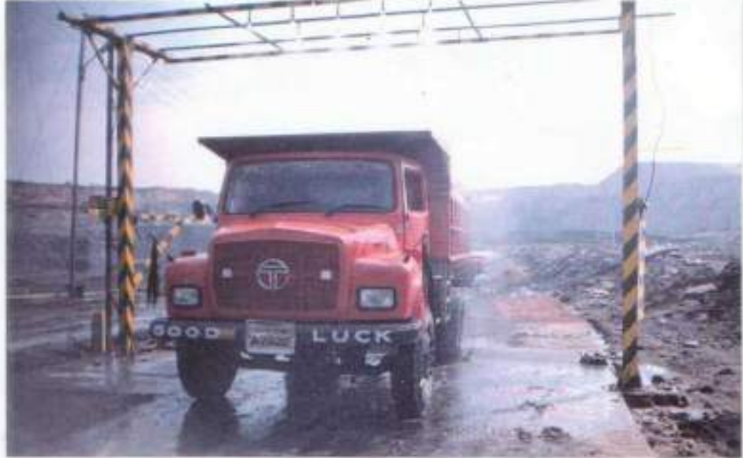
Fig. 7.8: Mechanism for showering water on dumpers
