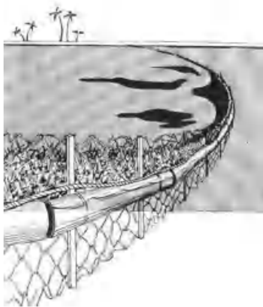
Fixed oil barrier constructed with straw bales and wire netting nailed to wooden stakes.
