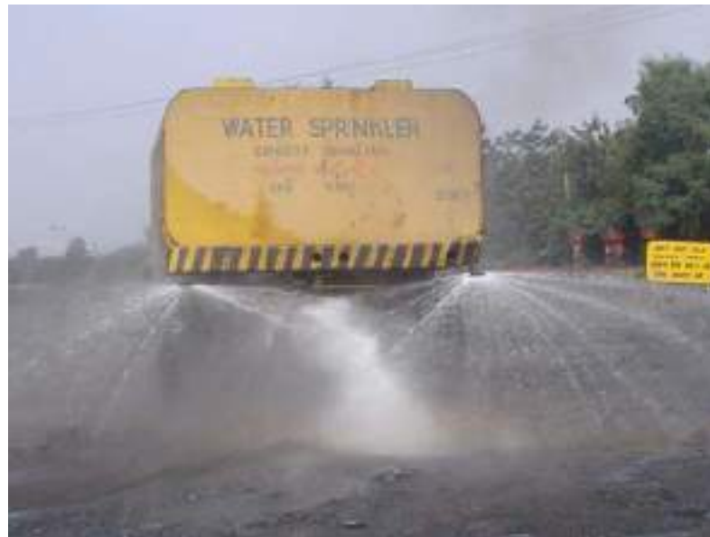
Fig. 7.10: Mobile water sprinklers
