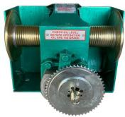
The Sustaining type double drum winch for high mast to be provided checking load to be carried for lowering down / raising up mechanism / maintenance cage operation. The double drum disc shall fulfil following technical parameters
