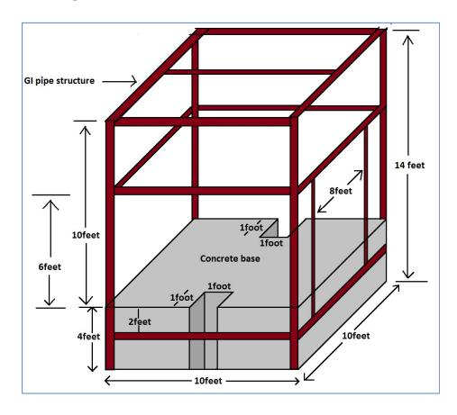
The figure includes only basic outline and the minimum structural features that must be included in the construction of the room. The concreting of base has to be done with mixture of 1:2:4 Cement:Sand:Metal and GI pipe structure
